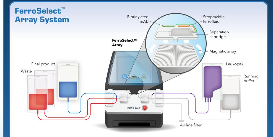
The FerroSelect Array is an automated, functionally closed, cell selection platform for process development and cell therapy manufacturing
